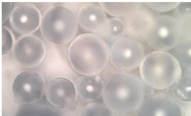
Figure 4. Improved 100% dense ADN prills with reduced sensitivity.
